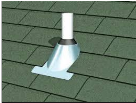
1.1 Item 2(Picture) Illustration of proper plumbing vent installation
