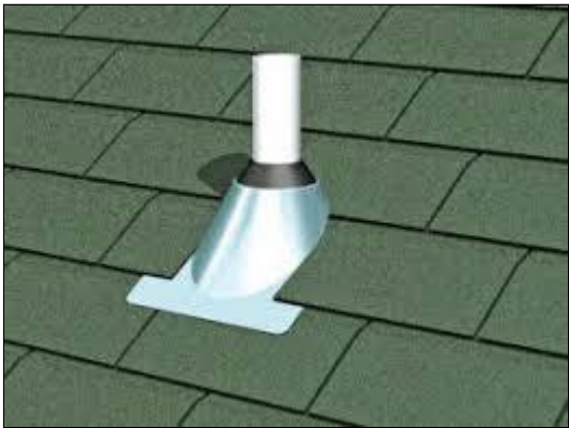
1.1 Item 2(Picture) Illustration of proper plumbing vent installation
